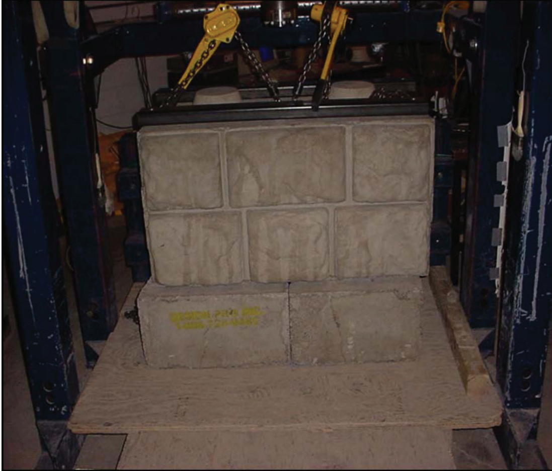
FIGURE 2: Photograph of World Block Landscape Block units in the connection test apparatus
